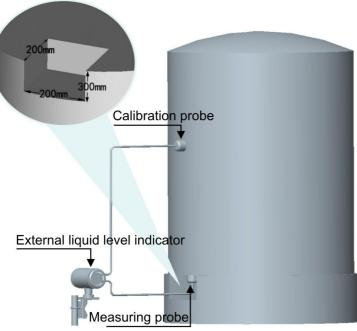
The measuring probe installation position must be remote from the input and exit pipes in the tank in order to avoid turbulent flow created by entrance or exit of liquid affecting the measurement.
